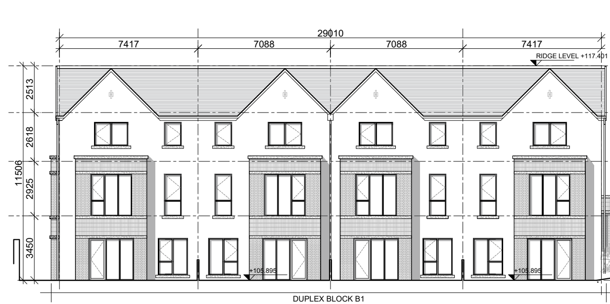
1 North Facing Elevation 0455
